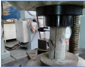
Fig. Mode of failure for the sandstone
